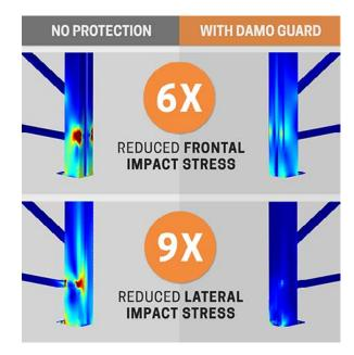
An impact study performed on an upright column showed that the DAMO GUARD decreases the stress on the original column by a factor of 6 on the front and by a factor of 9 on the sides.
